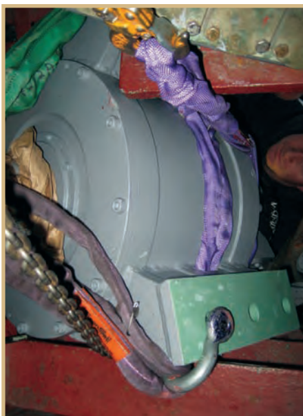
Right: The motor in drydock at Electric Boat, going through the grate. Left: The motor seen here with the bedplate obstruction.
