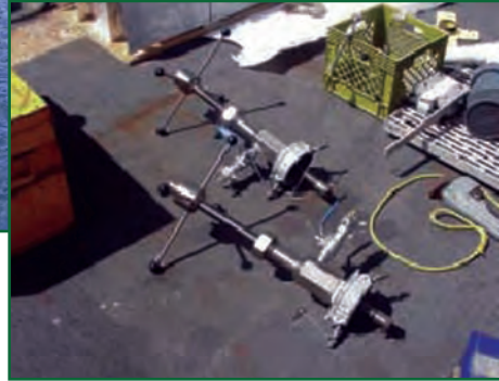
Left: Divers from MDSU 1, SWRMC, and pollution response experts from SUPSALV supporting the U.S. Coast Guard to assess the remaining petroleum products aboard the ex-USS CHEHALIS. Right: Two light weight hot tap systems shown, which will be the type of tool used during the offloading operation.
